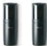
FT210 PAIR OF OPTICAL DEVICES FOR SENSITIVE EDGES FASTENED ON MOVING DOOR, CAN BE SWIVELLED THROUGH 210° WITH RELAY OUTPUT. BATTERY KIT (FTA1/FTA2) COMPULSORY.
